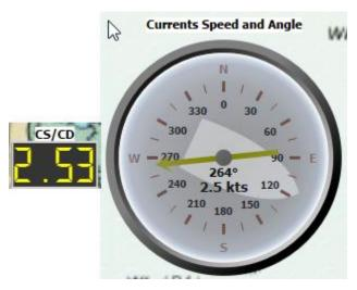
Currents Speed and Direction are either received from NMEA input, or calculated by qtVlm from COG, SOG, CTW and STW. Please note that Currents direction indicates where the Currents goes, contrary to Winds for which direction indicates where wind come from.
