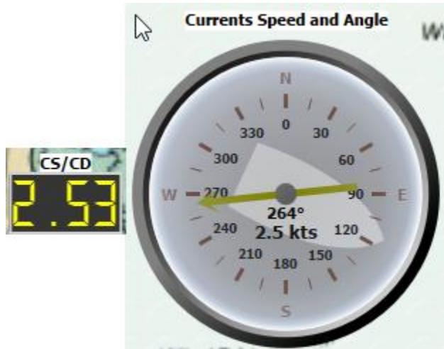
Currents Speed and Direction are either received from NMEA input, or calculated by qtVlm from COG, SOG, CTW and STW. Please note that Currents direction indicates where the Currents goes, contrary to Winds for which direction indicates where wind come from.
