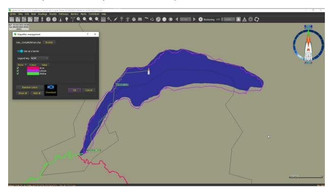
In the above example a shapefile is used instead of gshhs for detecting coasts at Lac Léman.
