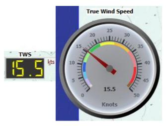
This instrument displays True Wind Speed. If NMEA data do not provide it and if it is possible, qtVlm will calculate it based on COG, SOG and apparent wind data.
