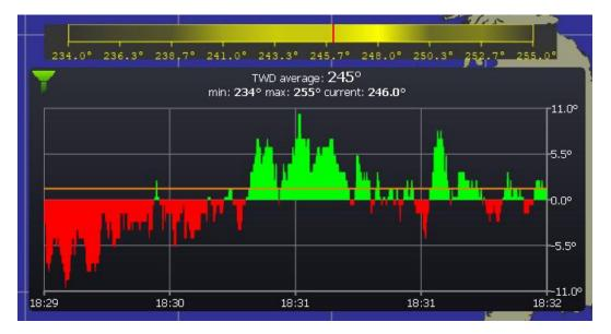
In the main instruments' configuration tab, you can also ask for "TWD distribution in TWD histogram". In that case the histogram will also show a band representing the statistical distribution of TWD (black means less occurrences, yellow means more occurrences).
