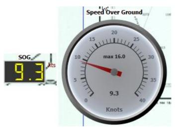
This instrument displays Speed Over Ground. The maximum speed reached is also displayed.
