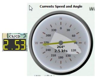
Currents Speed and Direction are either received from NMEA input, or calculated by qtVIm from COG, SOG, CTW and STW. Please note that Currents direction indicates where the Currents goes, contrary to Winds for which direction indicates where wind come from.
