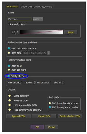
Max distance is the distance qtVlm will check from the pathway for dangers (orange) or obstacles (red). It will try to shrink the safe path until it reaches the Min distance, declaring it red (grounding alert).
