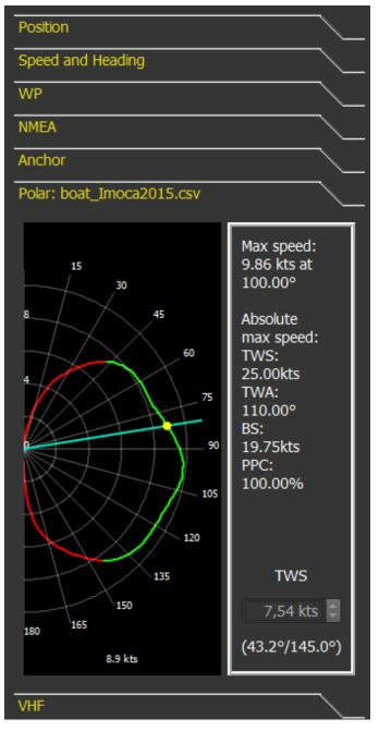
This tab shows boat polar and display best wind angle upwind and downwind (left image).
