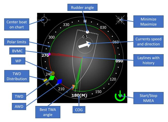
TWD indicator will be either green or red, depending on polar limits. The rudder scale is limited to -30°/+30° and the indicator will smoothly turn red when approaching 30° rudder angle.
