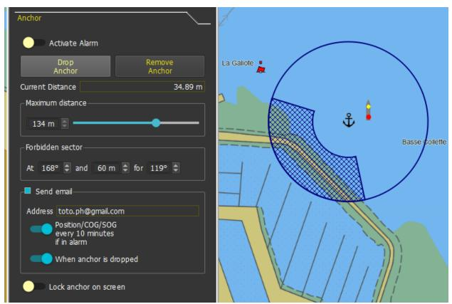
This manages Anchor Alarm. Anchor is also moveable with mouse, unless specifically locked on screen.
