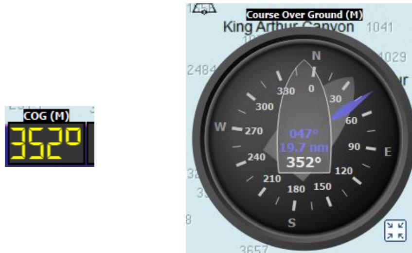
This instrument displays Course Over Ground, plus heading/distance to WP (in blue). The background boat shape is oriented according to CTW.
