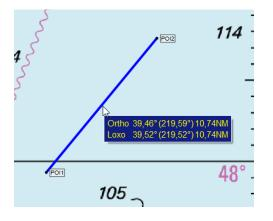
This function can also be used to find the position of an object, by placing several such lines. Place the first POI on the boat and the second one in the measured bearing of the object and repeat the operation several times when the boat has moved enough. The object approximate position will be where the lines are crossing. Useful for instance to find the position of a mark during racing.
