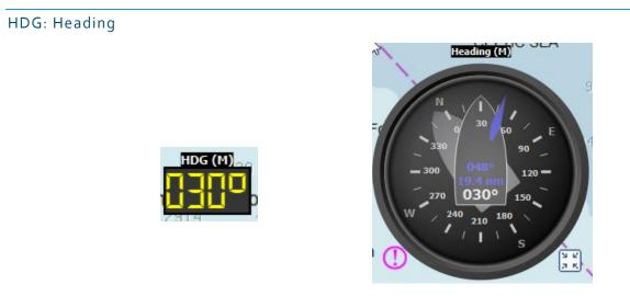
This instrument shows heading as measured on a Compass. It is different from COG in case of Currents, for instance. It also displays heading/distance toward current waypoint (in blue). The background boat shape is oriented according to COG.
