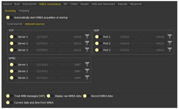
This configuration screen is available via menu "qtVlm->Configuration" and allows to configure NMEA connections. Using several connections simultaneously is allowed.
