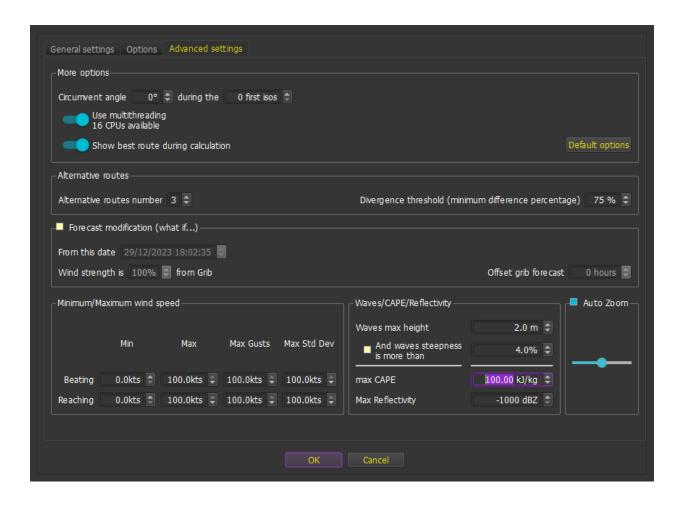
• <u>Circumvent angle</u>: this option can be useful when the destination is completely obfuscated by an obstacle and the boat is too close from it for the routing to find a solution. In that case you can help it by specifying a deviation angle for the few first isochrons.
