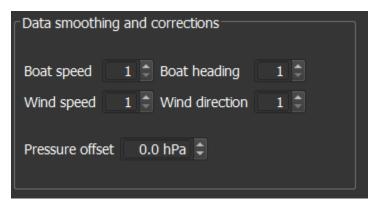
It is possible to smooth data received for wind speed and direction, and boat speed and direction. The value indicates the number of last received data that should be averaged. As these data are used in all calculations, it allows to carefully tune the sensibility of instruments, for instance Polar Efficiency Percentage (PPC). The default value (1) means not smoothing.
