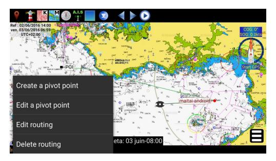
« *Create a pivot point* » will simply restart the routing there, continuing toward the same arrival. « *Edit a pivot point* » allows to edit the routing before, essentially to change arrival point. This function is useful to force passage points, or even to manage U-turns.
