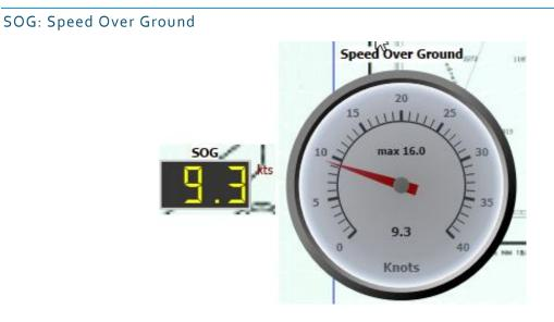
This instrument displays Speed Over Ground. The maximum speed reached is also displayed.
