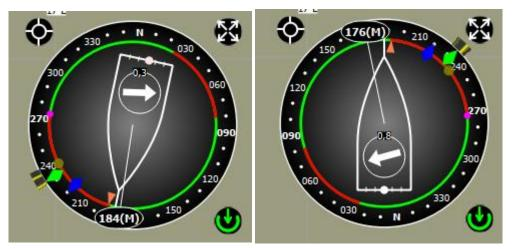
Tactical Microboard shows much more data than VLM microboard. It can be oriented North-Up or Bow-Up and can show laylines on active WP.
