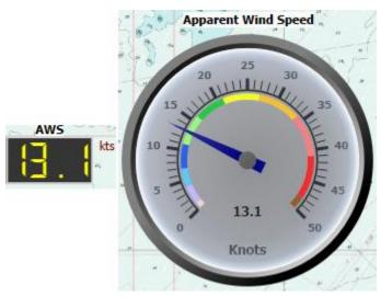
This instrument displays Apparent Wind Speed. If NMEA data do not provide it and if it is possible, qtVlm will calculate it based on COG, SOG and real wind data.
