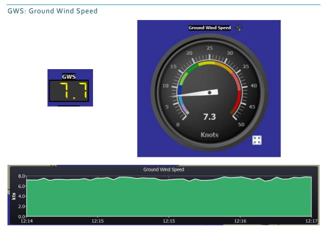
This instrument displays Ground Wind Speed, which is the vector subtraction of Sea Wind (TWS/TWD) and currents.
