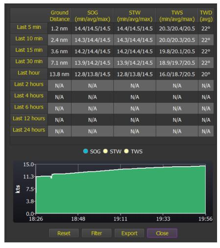
The save button exports all collected data in CSV format. Filter button removes abnormal values based on standard deviation.
