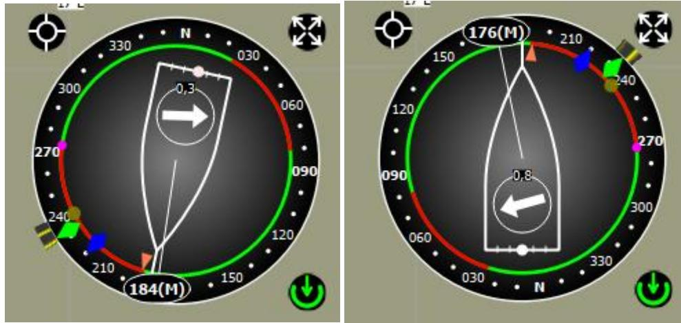
Tactical Microboard shows much more data than VLM microboard. It can be oriented North-Up or Bow-Up and can show laylines on active WP.
