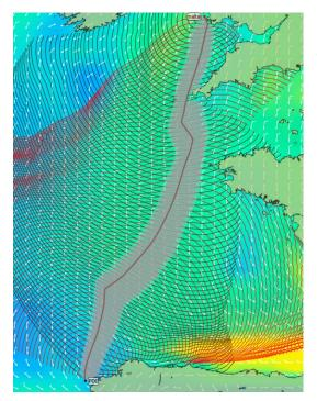
On this image, envelope is regular and large enough. The routing is probably stable and reliable.
