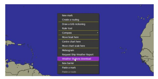
Stations reports will be downloaded in a range from the mouse position, by default 300 NM. This default can be changed in the grib configuration tab of the main settings.
