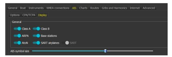
Options controlling CPA (Closest Point of Approach) and TCPA (time to CPA) allows to configure alarms (sound and/or visual). Real boat sizes can be used for these calculations. These calculations can be deactivated completely.
