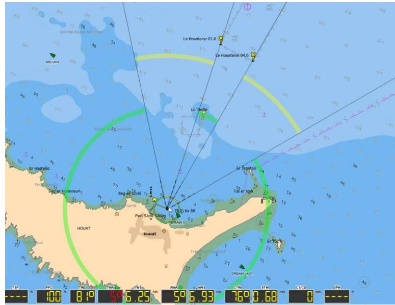
The lighthouse icon in the toolbar has three states: Lights hidden, lights shown, and lights visible from boat:
