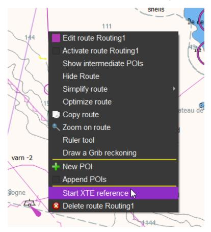
Once an XTE reference is defined, a small dashed line will appear that represents the track that was planned. The distance to this line is shown in the XTE instrument, and the position where the boat should be on this track is also shown.
