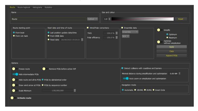
Several options are available, including most important starting point and starting date. You can also choose to show or not intermediate POIs, or to detect collision with land and barriers. You can alter grib data from grib and play with polar efficiency individually for this route.
