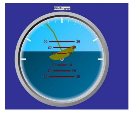
The "mast-needle" is articulated so it shows the correct heel graduation whatever the height of boat and water.
