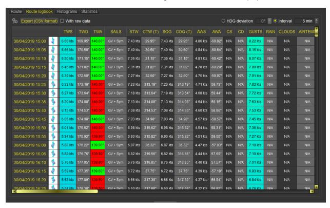
**Warning**: Winds information at route level includes wind generated by Currents, if this data is available in gribs. Consequently, wind data in route's log might differ from pure wind grib data.
