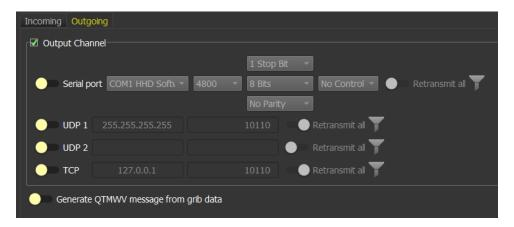
The output channel is used to send current WP information to a navigation system. It can also be used to send performance data to NKE instruments. There is also an option for retransmitting all NMEA data on a port.
