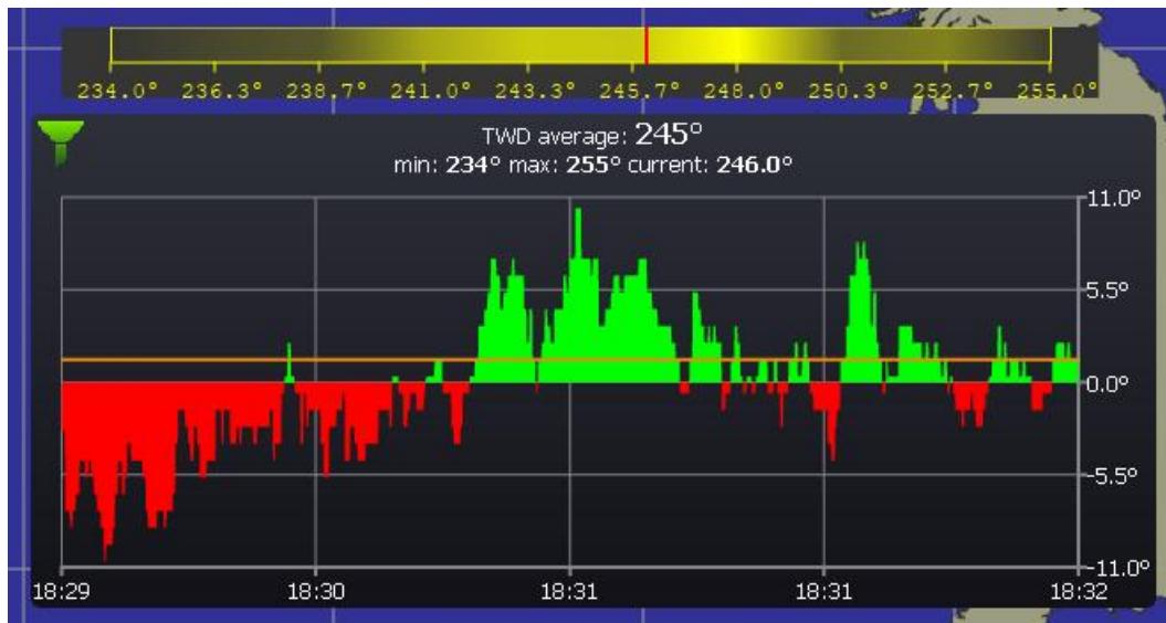
In the main instruments' configuration tab, you can also ask for "TWD distribution in TWD histogram". In that case the histogram will also show a band representing the statistical distribution of TWD (black means less occurrences, yellow means more occurrences).
