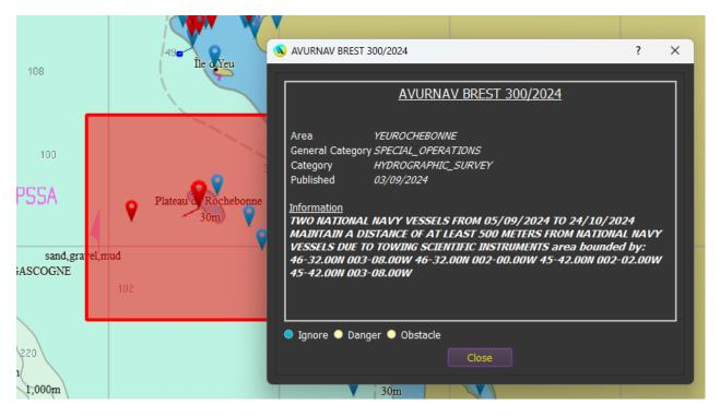
Note that you can define an Avurnav as an obstacle or a danger. An obstacle will be avoided by routings and routes, while a danger will trigger various alarms.
