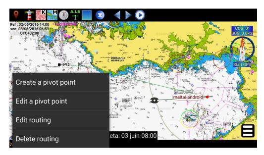
« *Create a pivot point* » will simply restart the routing there, continuing toward the same arrival. « *Edit a pivot point* » allows to edit the routing before, essentially to change arrival point (Edit a pivot is not possible if routing on a pathway). This function is useful to force passage points, or even to manage U-turns.
