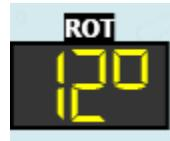
This instrument shows the boat's rotation angle per minute.
