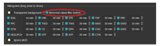
In that case a filter button will be displayed in each histogram, which when press will remove any abnormal values (if any), based on a standard deviation formula.
