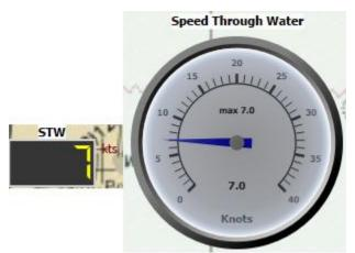
This instrument shows Speed Through Water. It is different from SOG in case of Currents, for instance. It also displays the maximum value measured.
