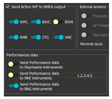
qtVIm can send performances sentences on NMEA output port, to be displayed on NKE or Raymarine instruments. These data consist in theoretical polar speed, opposite track heading with the same TWA, target speeds for CMG and VMG, optimum polar angles for upwind and downwind, and currents direction and speed calculated by qtVIm (based on COG, SOG, CTW, STW).
