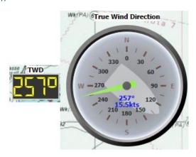
This instrument shows True Wind Direction. If NMEA data do not provide it and if it is possible, qtVlm will calculate it based on COG, SOG and apparent wind data. The arrow's color changes with wind speed, and boat orientation is drawn on background.
