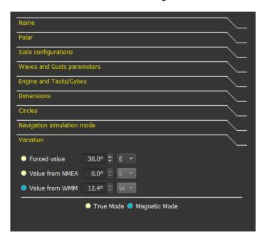
Instruments will use this data is (M) mode is selected. You can either use a forced value or get the magnetic variation from NMEA message (RMC), or from WMM (World Magnetic Model).
