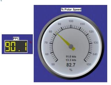
This instrument shows the difference between actual speed and theoretical polar speed, as a percentage and as values. It is also possible to send this data through the NMEA output port in order to display it on NKE or Raymarine instruments.
