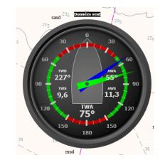
This instrument shows True Wind Angle. If NMEA data do not provide it and if it is possible, qtVlm will calculate it based on COG, SOG and apparent wind data. The value and the arrow are green when TWA is inside the polar VMG limits, red otherwise. The digital display also shows a red or green dot, depending on the tack. The red parts on the dial represent the polar VMG limits and are recomputed dynamically.
