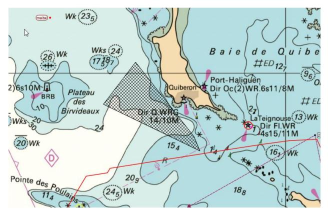
Barriers are used by Weather Routing Module and Routes Module. They can be used to force a passage, to define a No Sailing Zone, etc.
