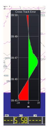
This instrument shows the distance between your position and a theoretical route, in meters. An XTE reference must have been defined, this is done through the route contextual menu. XTE reference can be deleted from the route menu. See <u>Routes Module</u> for more information.
