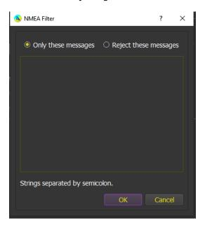
Message to be treated by the filter must be separated by semi column. For instance, if you want to filter all AIS messages just a "!" is enough in the list of strings.
