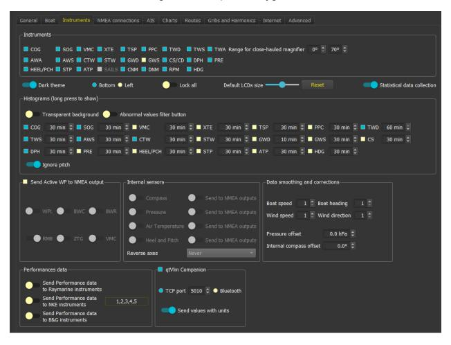
Each instrument is made of an **LCD** plus eventually a **dial** and eventually a **histogram**. The size of the digital displays can be adjusted in the configuration dialog, General tab. The dial is displayed/hidden by **pressing shortly** on the digital display, and the histogram by a **long press**. It is recommended to activate only histograms you really need since histograms are quite costly resources wise.
