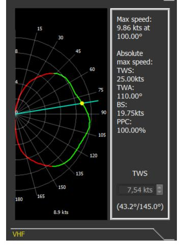
This tab shows boat polar and display best wind angle upwind and downwind (left image).
