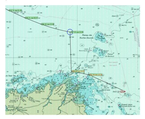
Some POIs will appear in red. These POI are non-simplifiable points, generated by routing, and that cannot be removed or moved because they are useful to avoid coats or barriers.
