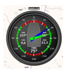
This instrument shows True Wind Angle. If NMEA data do not provide it and if it is possible, qtVlm will calculate it based on COG, SOG and apparent wind data. The value and the arrow are green when TWA is inside the polar VMG limits, red otherwise. The digital display also shows a red or green dot, depending on the tack. The red parts on the dial represent the polar VMG limits and are recomputed dynamically.
