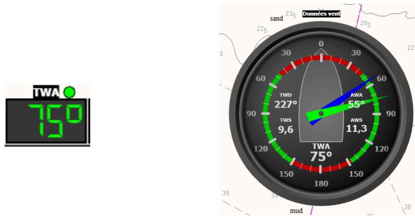
This instrument shows True Wind Angle. If NMEA data do not provide it and if it is possible, qtVlm will calculate it based on COG, SOG and apparent wind data. The value and the arrow are green when TWA is inside the polar VMG limits, red otherwise. The digital display also shows a red or green dot, depending on the tack. The red parts on the dial represent the polar VMG limits and are recomputed dynamically.
