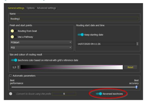
This function calculates inversed isochrons, i.e. it starts from arrival point and date and calculates from where it could have come to be there and starts again until it reaches starting point. This calculation allows to determine an envelope where regular and inversed isochrons are crossing. This envelop shows where the passage would be equivalent. A thin envelope is a clear sign that there is uncertainty in the routing because the passage found might well disappear on the next grib update.
