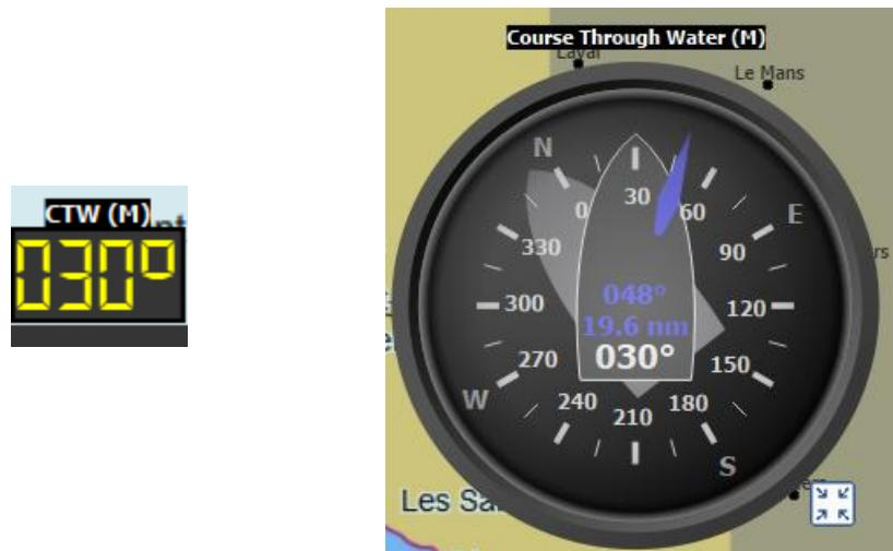
This instrument shows Course Through Water. It is different from COG in case of Currents, for instance. It also displays heading/distance toward current waypoint (in blue). The background boat shape is oriented according to COG.
