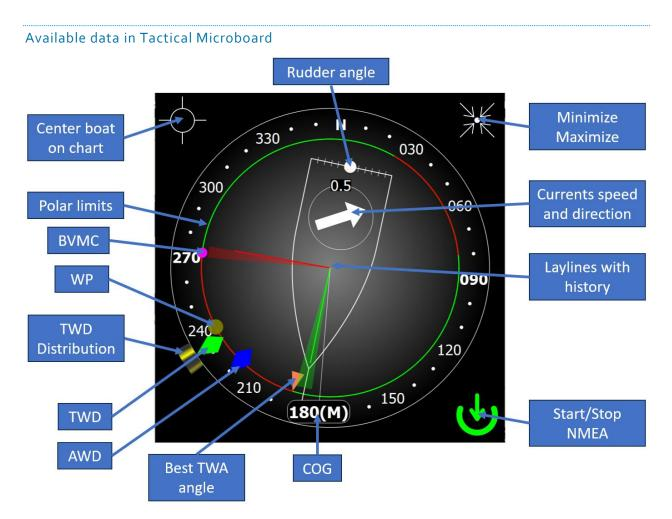
TWD indicator will be either green or red, depending on polar limits. The rudder scale is limited to - 30°/+30° and the indicator will smoothly turn red when approaching 30° rudder angle.
