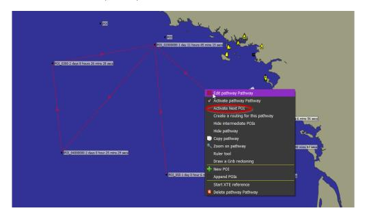
Contrary to routes which calculate ETAs based on boat's polar and grib data, pathways compute ETAs based on actual boat speed, or based on speed that have been input in the Information and management tab. It is therefore convenient when motoring.
