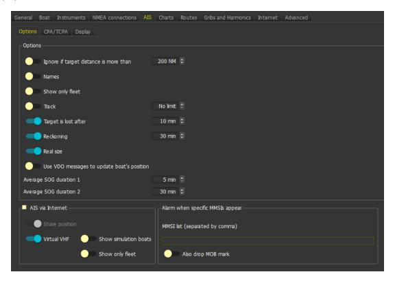
The first option filters out targets based on their distance to boat.
