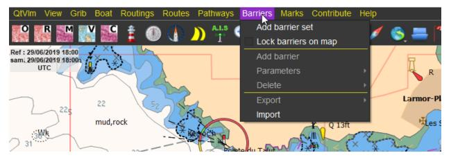
Barriers are positioned with mouse or finger. Once placed you can move points, add/remove points, close the barrier, etc.
