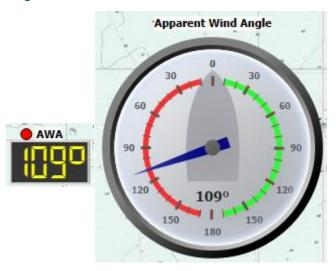
This instrument displays Apparent Wind Angle. If NMEA data do not provide it and if it is possible, qtVlm will calculate it based on COG, SOG and real wind data.
