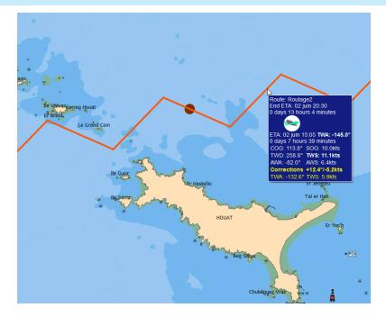
A big dot appears on the route when the grib date is moved forward. This corresponds to the position of the boat at that date. It can also be seen when animating gribs.
