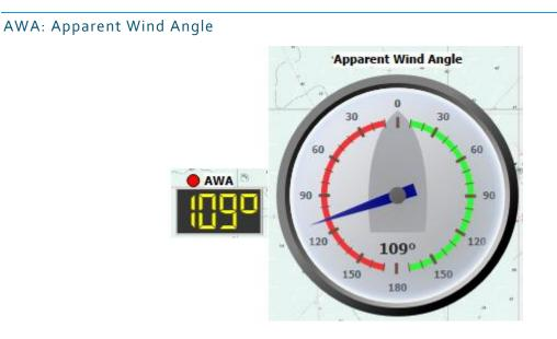
This instrument displays Apparent Wind Angle. If NMEA data do not provide it and if it is possible, qtVlm will calculate it based on COG, SOG and real wind data.
