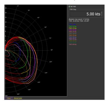
This dialog shows critical angles for the polar (best VMGs). Note that it is possible to modify the polar outside qtVlm in the same time. Just press "Reload polar" each time you save it.
