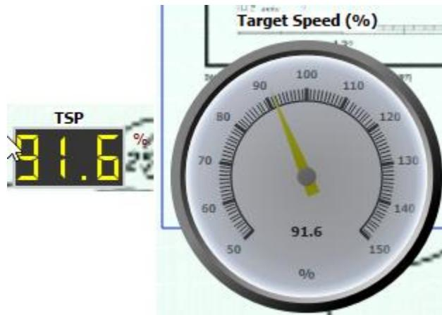
This instrument expresses the speed (STW) in percentage of optimum speed as given by the polar to reach the WP. Optimum speed is the speed on water corresponding to the best VMC towards the WP. For instance, for a WP upwind, too much speed means you must luff up a bit, while a percentage lower than 100% means you must bear away a bit. For steering, this information is often more efficient than VMC
