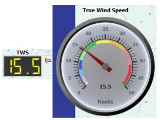
This instrument displays True Wind Speed. If NMEA data do not provide it and if it is possible, qtVlm will calculate it based on COG, SOG and apparent wind data.
