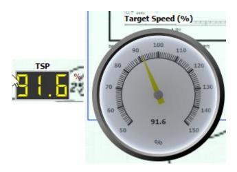
This instrument expresses the speed (STW) in percentage of optimum speed as given by the polar to reach the WP. Optimum speed is the speed on water corresponding to the best VMC towards the WP. For instance, for a WP upwind, too much speed means you must luff up a bit, while a percentage lower than 100% means you must bear away a bit. For steering, this information is often more efficient than VMC
