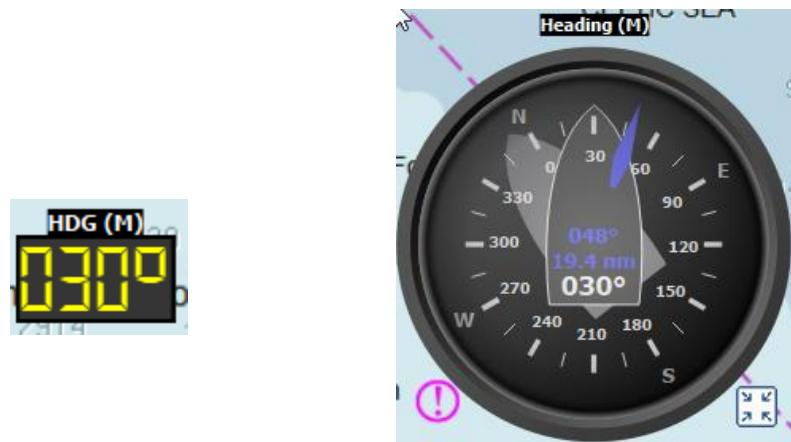
This instrument shows heading as measured on a Compass. It is different from COG in case of Currents, for instance. It also displays heading/distance toward current waypoint (in blue). The background boat shape is oriented according to COG.
