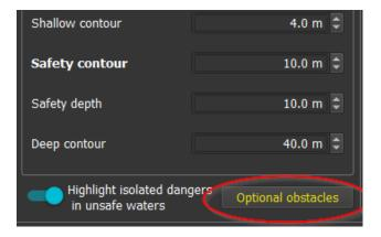
Safety Contour parameter in charts parameters is particularly important. It is used to identify Depth Contours that will be drawn with a thicker line. Please note that if there is no Contour Depth matching exactly your setting, the next Contour Depth object will be used unless the next Contour Depth object as a depth more than 67% if setting is <= 10m or 33% if > 10m. In that case a default Safety Control will be drawn. Safety contour is a danger, but not an obstacle.
