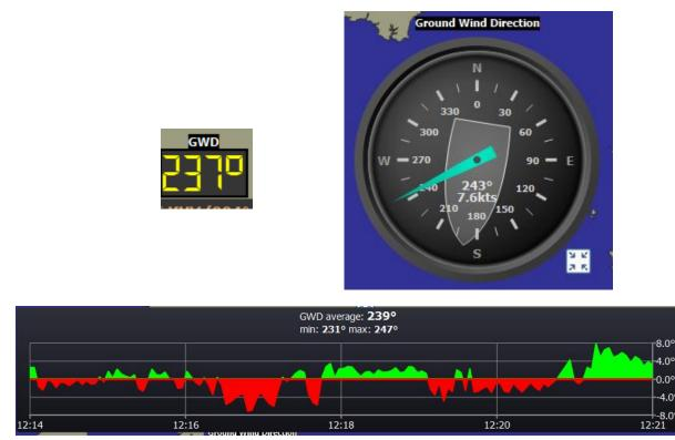
This instrument shows Ground Wind Direction, which is the wind blowing on Earth as opposed to TWS/TWD which is the wind blowing on the sea.
