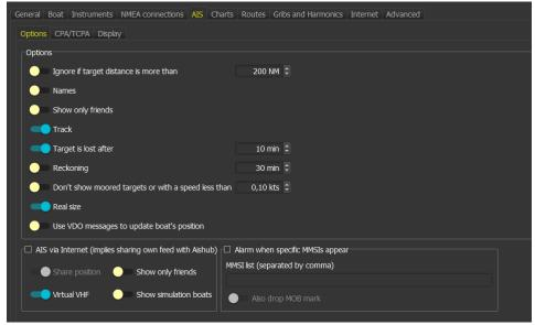
A simulation mode is proposed in qtVlm, through a collaboration with **sinagot.net** and **AisHub.com**. It receives real AIS targets via Internet, and allows to simulate sailing between them, using gribs data and polar to move the boat. This mode is accessible via the menu "Boat->Simulation mode".
