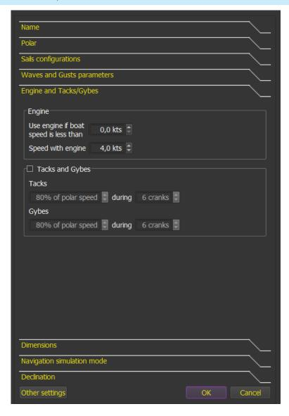
You can specify that when the boat's speed with sails is under a value, the engine is started, with a boat's speed in that case that will override the polar value. Note that if any waves parameter is setup, the engine's speed will be affected by these parameters.
