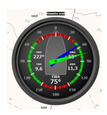
This instrument shows True Wind Angle. If NMEA data do not provide it and if it is possible, qtVlm will calculate it based on COG, SOG and apparent wind data. The value and the arrow are green when TWA is inside the polar VMG limits, red otherwise. The digital display also shows a red or green dot, depending on the tack. The red parts on the dial represent the polar VMG limits and are recomputed dynamically.
