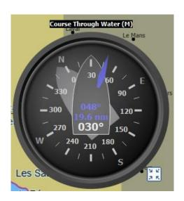
This instrument shows Course Through Water. It is different from COG in case of Currents, for instance. It also displays heading/distance toward current waypoint (in blue). The background boat shape is oriented according to COG.
