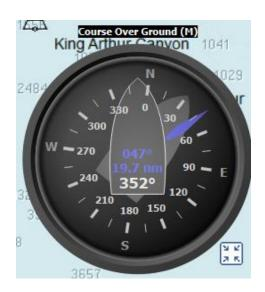
This instrument displays Course Over Ground, plus heading/distance to WP (in blue). The background boat shape is oriented according to CTW.
