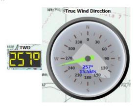
This instrument shows True Wind Direction. If NMEA data do not provide it and if it is possible, qtVlm will calculate it based on COG, SOG and apparent wind data. The arrow's color changes with wind speed, and boat orientation is drawn on background.
