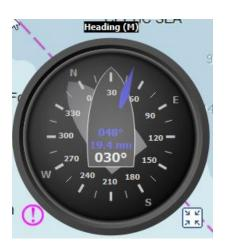
This instrument shows heading as measured on a Compass. It is different from COG in case of Currents, for instance. It also displays heading/distance toward current waypoint (in blue). The background boat shape is oriented according to COG.
